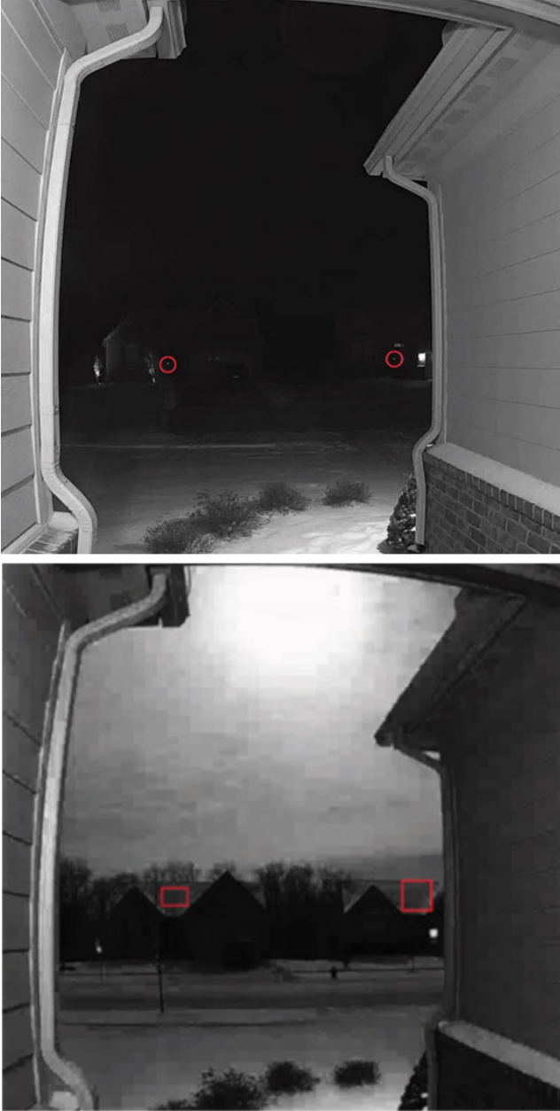
Fig. 6. Screen capture of two frames of Ypsilanti, Michigan, video showing regions used for relative brightness (square regions—bottom) changes and calibration light sources (circled—top). Image credit Daniel McGhee.
