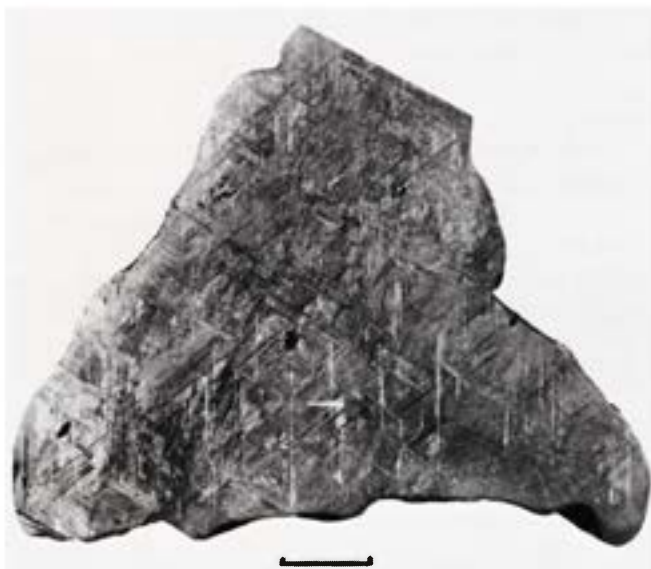
Figure 1339. Otchinjau (Brit. Mus. no. 1953, 61). A 1,450 g sample showing the structure of a fine octahedrite of group IVA. Deep-etched. Scale bar approximately 3 cm. Brit. Mus. neg. 8387.
