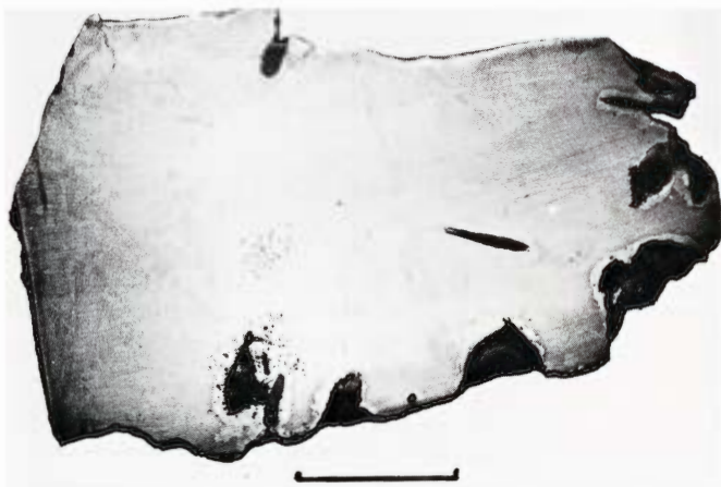
Figure 1327. Opava (Prague no. 322 of 68 g). A little known hexahedrite. The white zones along the rim and around troilite inclusions are artificial and represent metal that was protected by wax during deep-etching. Scale bar 2 cm.
