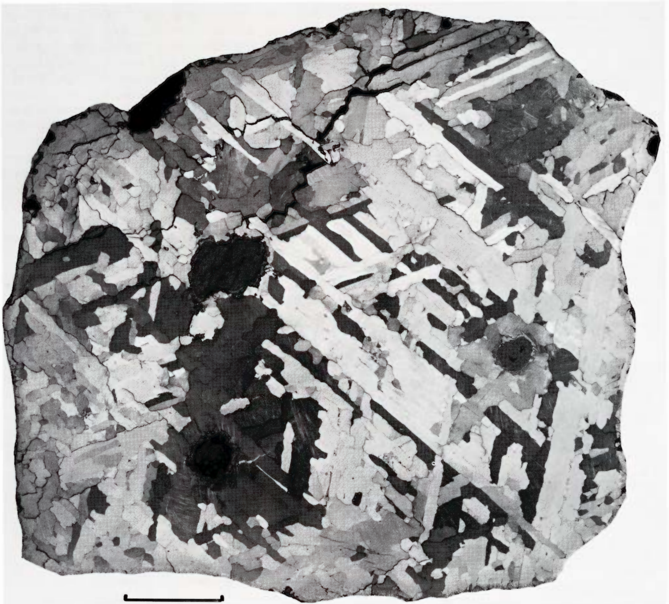
Figure 1338. Osseo (U.S.N.M. no. 925). A coarse octahedrite of group I. Three troilite-graphite nodules with schreibersite-cohenite rims. Deep-etched. Scale bar 30 mm. S.I. neg. 1641B.
