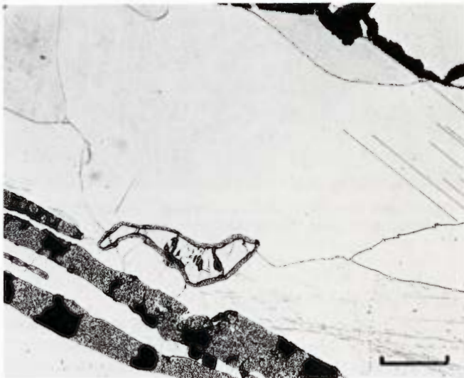
Figure 1335. Oscuro Mountains. Detail of Figure 1332. Below, two altered taenite lamellae. Above these, a schreibersite crystal (white) surrounded by fine blebs of taenite. Etched. Scale bar 150 \mu . (Perry 1950: Volume 7.)
