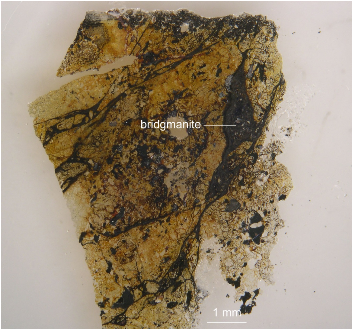
Fig. S5. An optical image showing Tenham thin section USNM 7703 where bridgmanite was identified in a shock vein. The shock melt veins are dark brown to black over the thickness of the thin section of about 30 \mu\text{m} .
