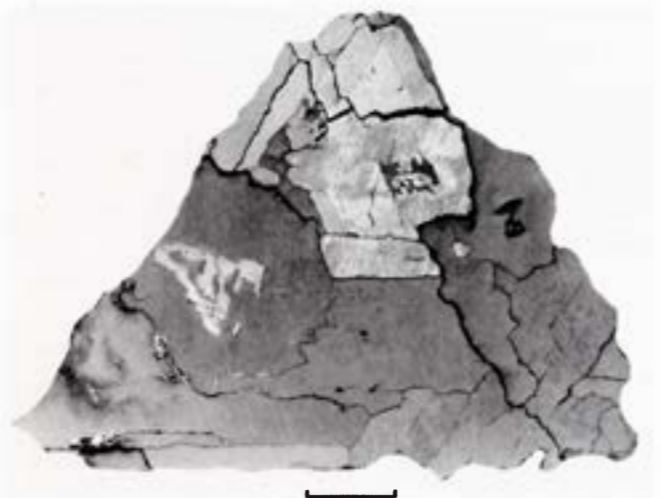
Figure 234. Ainsworth (U.S.N.M. no. 375). Coarsest octahedrite, group IIB. Large skeleton crystals of schreibersite enveloped in swathing kamacite. Etched. Scale bar 20 mm. S.I. Neg. 1517B.
