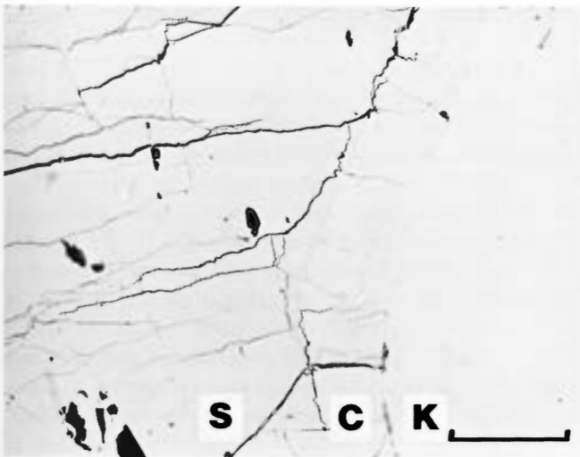
Figure 239. Enlarged area of Figure 238. Schreibersite (S), cohenite (C) and kamacite (K). Polished. Scale bar 100 \mu .
