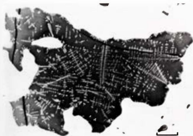
Figure 233. Typical slag inclusion in wrought iron, in this case from a Danish fifteenth century naval gun. Similar slags are present in Agricultural College and prove that it is a pseudometeorite. Polished. Scale bar 50 \mu .
