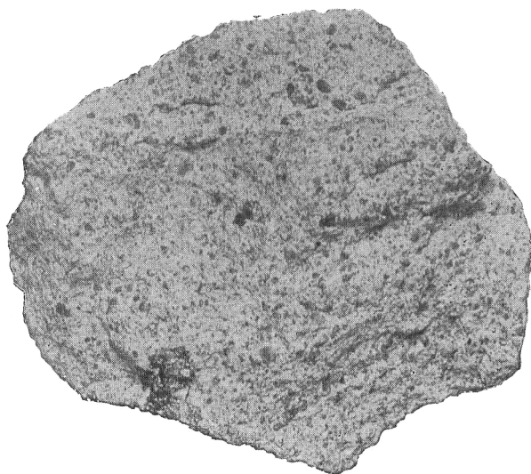
FIG. 13. Fractured surface with pyrrhotite nodule. \times 1 diameters.
